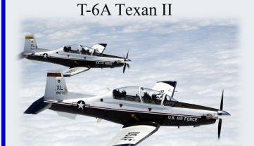
The T-6A Texan II is a single-engine, two-seat primary trainer designed to train Specialized Undergraduate Pilot Training students in basic flying skills common to U.S. Air Force and Navy pilots.
